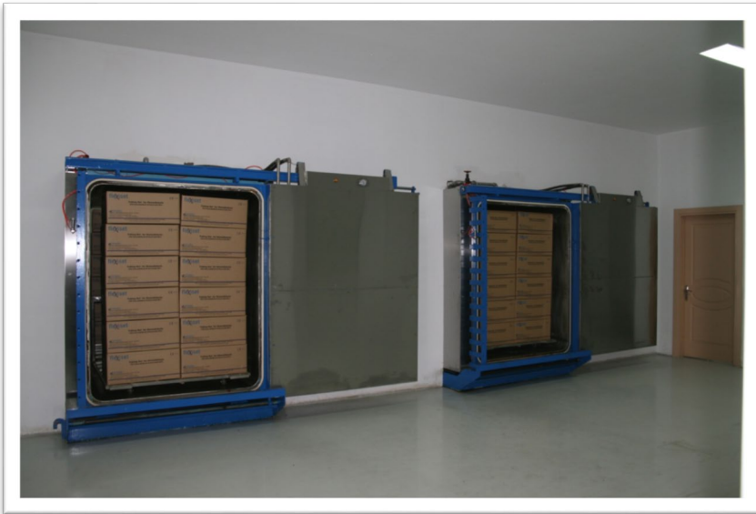
New ETO Sterilization System with Scrubber Unit for waste gas scavenging and recycling.
